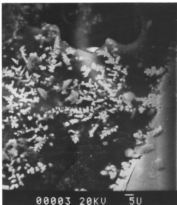
Fig. 3. Ag-Cu alloy powder mounted in acrylic resin and sectioned. The numerals indicate locations of EDX analyses and should be read in conjunction with Table 3.
