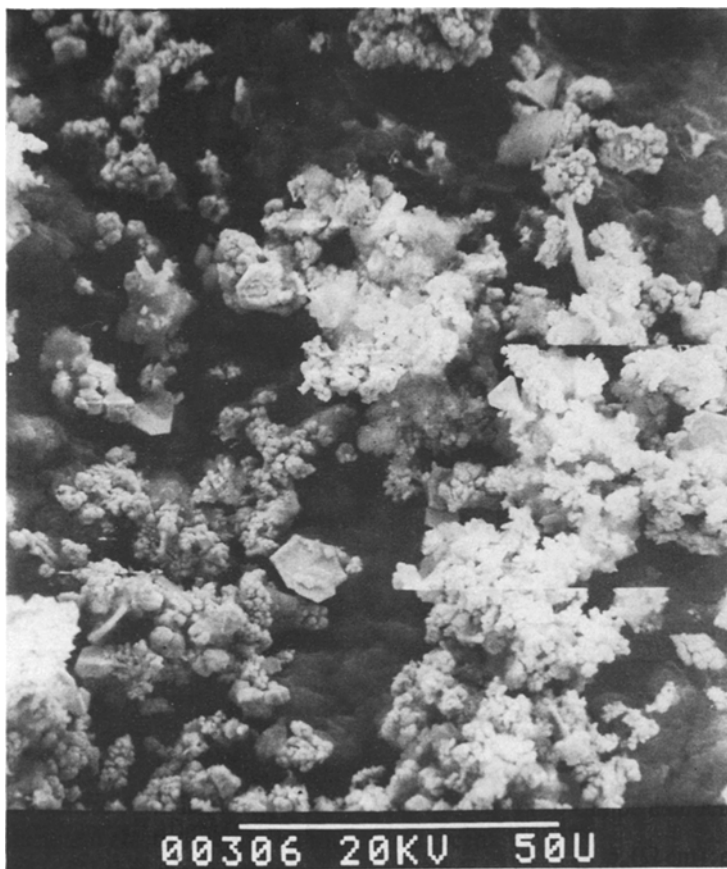
Fig. 1. Ag–Cu powder (60 Ag–40 Cu) produced from ammoniacal solution, and showing both nodular and tabular morphologies.
